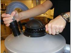
2. Block the suction hose by the work place. Wait about 7-10 sec. while the machine builds up a vacuum.
