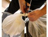
2. Cut between the cable ties.
