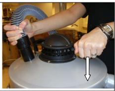
3. Press the filter cleaning valve hard
